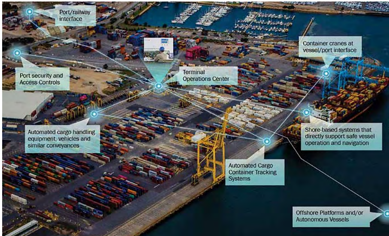
Figure 1. Example of the Interconnected Systems at a Container Terminal 5
